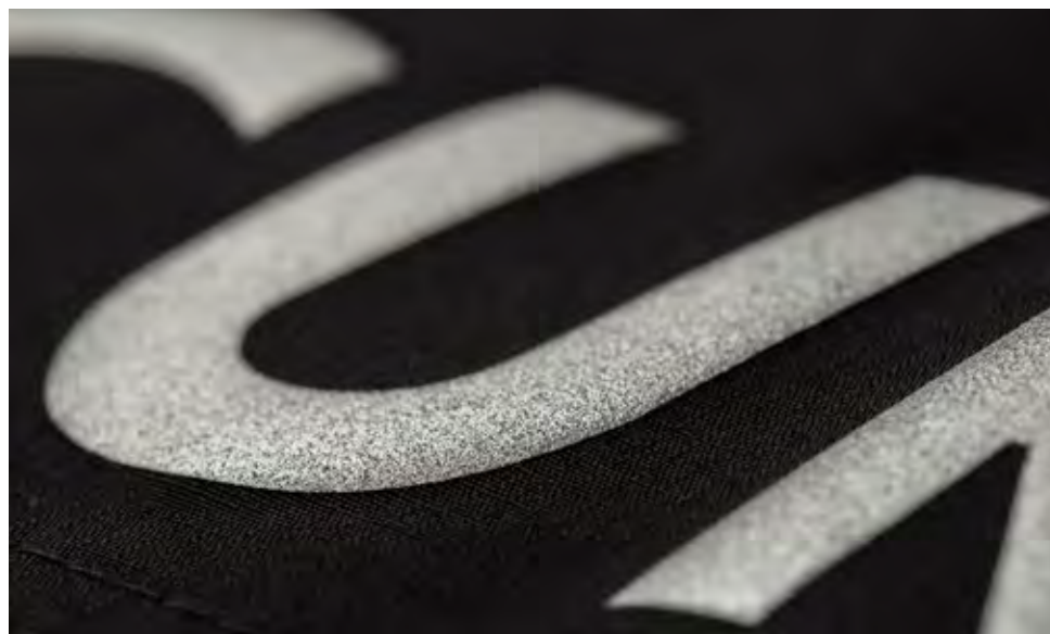
Transfer termosaldato riflettente. Heat-sealed reflective transfer.
